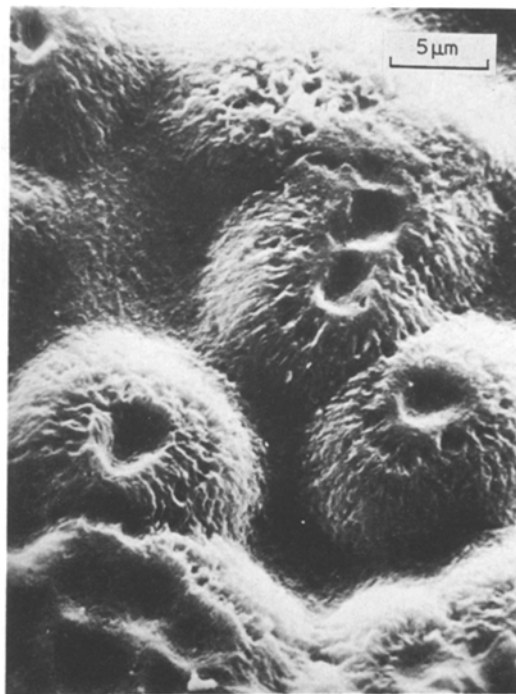
Figure 3 A selection of spherulites in the undeformed, etched polyethylene.
